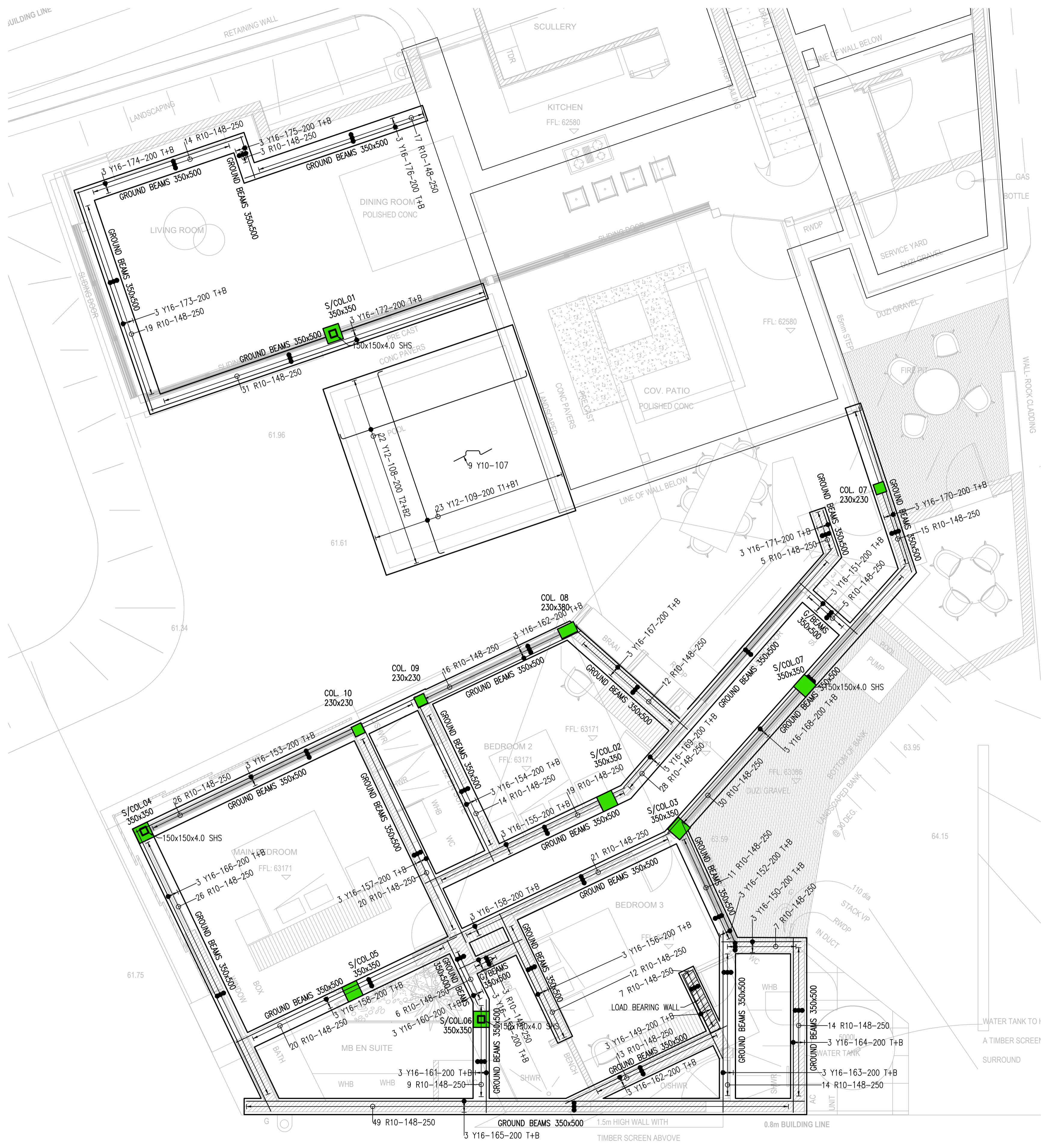
29.14m Boundary line 110 DIA UPVC SEWER PIPE @ MAX FALL 1:3 TO BE ENCASED IN CONCRETE UNDER DRIVEWAY REINFORCING DETAILS: UPPER GROUND BEAMS 1:50
