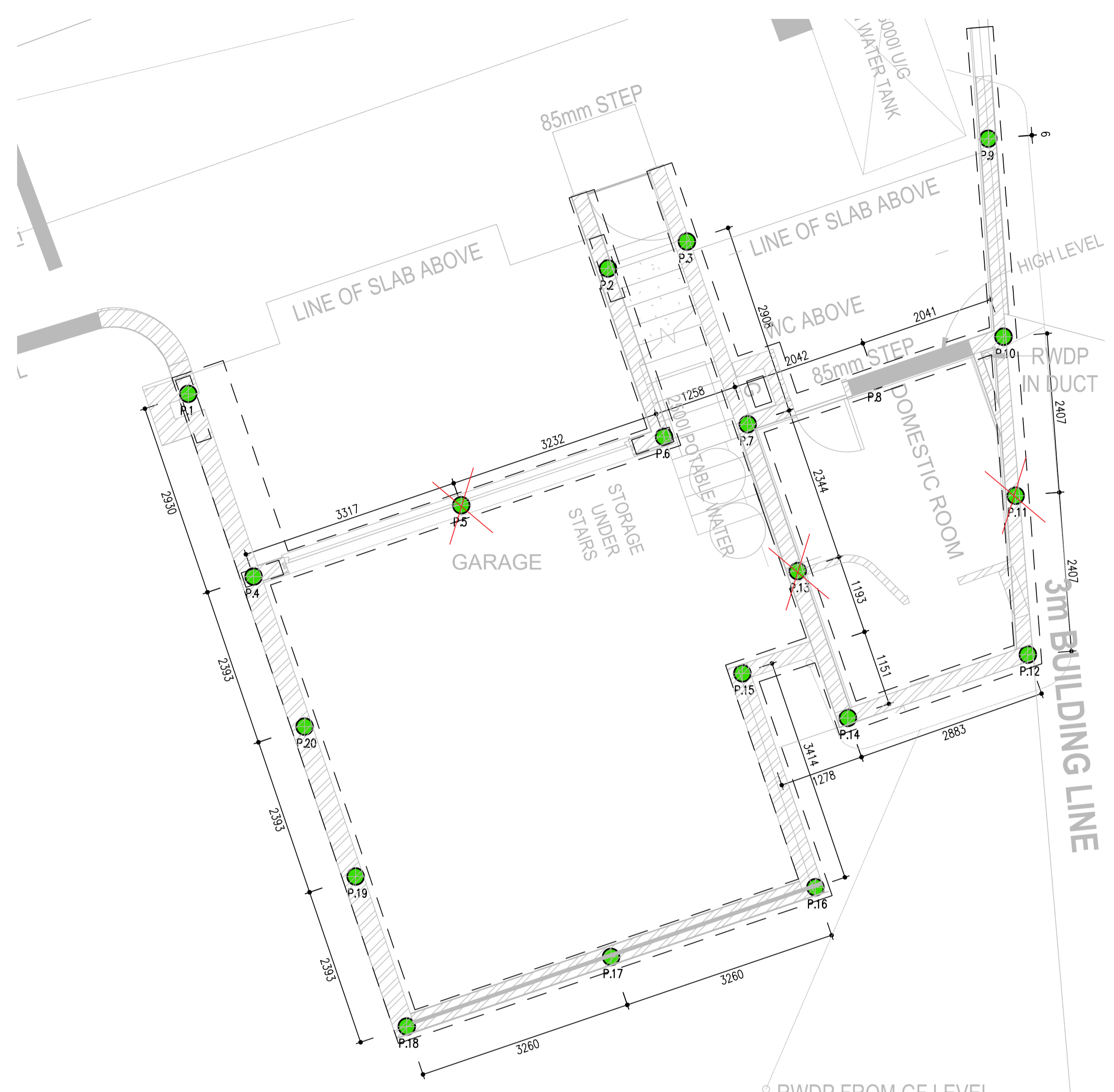
LOWER PILING LAYOUT 1:50
