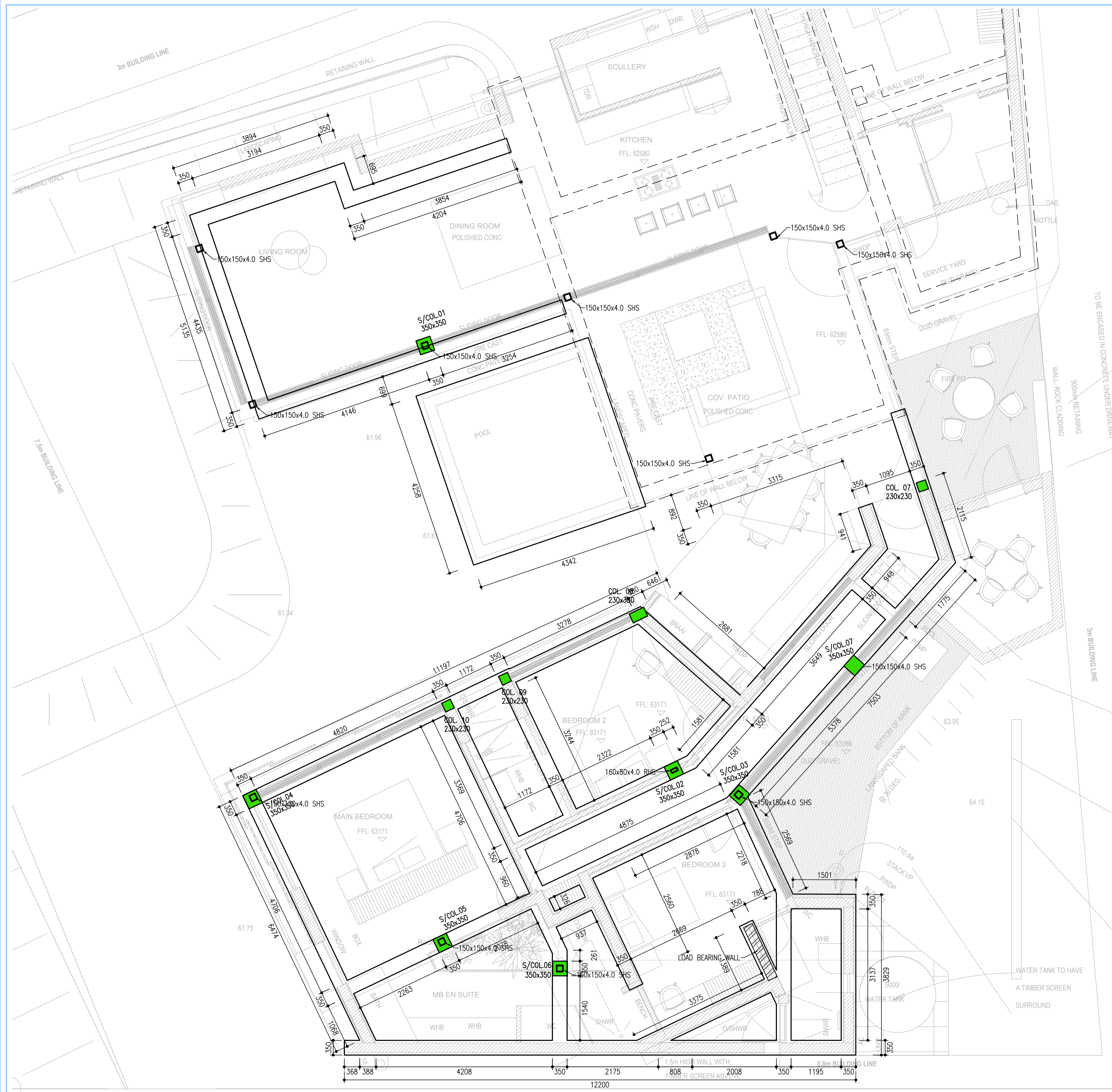
CONCRETE DETAILS: UPPER GROUND BEAMS 1:50
